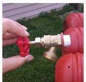
Wrap the spigot with plumber's tape and place a rubber washer flush against the base of the threads.
