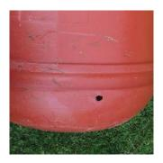
Using the  $\frac{3}{4}$ " wingbit, drill a hole about 6-8" from the bottom of the barrel.
