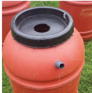
Use the 4" hole saw to drill a hole in the lid of the barrel. Drill slowly and with caution, as a 4" hole saw creates lots of torque—drilling too quickly could cause damage to the barrel or to you.
