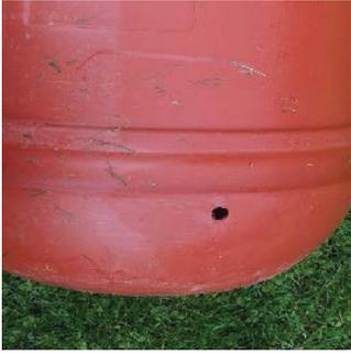
Using the 3/4" wingbit, drill a hole about 6-8" from the bottom of the barrel.
